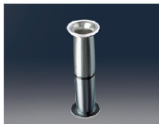
압확시험 [Flaring Test]
